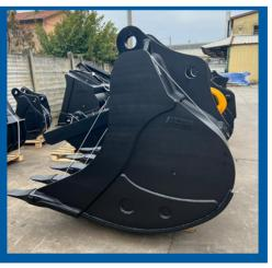
Abrasion adapters have a thicker upper leg, providing excellent abrasion resistance. In addition, the PR shape has a good tooth profile, which ensures a strong penetration. This shape is a good compromise between wear material and penetration.
