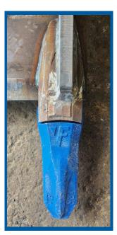
The PR shape has a good tooth profile, which ensures a strong penetration. This shape is an excellent compromise between wear material and penetration.
