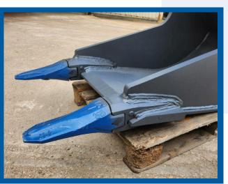
The customer was looking for an innovative and safe system for breaking materials at elevated heights. As an alternative to the ripper tooth, the customer chose this type of 2-teeth bucket.
