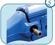
Pin insertion: Once the teeth is correctly Pin insertion (2): Before pin clamping, installed on the adapter, insert TK13CL® the pin should be in "head down" pin into the key hole while respecting the insertion direction (pin head down), then push it to the end.
