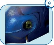
Correct locking: After the "clac" sound, the pin will be locked as shown. The pin rotation is fully completed, the pin cannot be turned any further.
