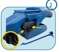
Sleeve insertion: Manually insert the sleeve. You will notice on the sleeve & the adapters some notches to make sure to respect the sleeve insertion direction.
