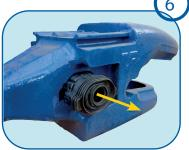
Sleeve removal (2): Once the plug is partially removed, you can complete removal manually.
