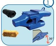
Cleaning: Tilt the bucket 30° upwards. Before inserting turnkey sleeve in its housing, we recommend to clean the adapter sleeve housing as well as the adapter nose to make sure the sleeve will be correctly positioned into the sleeve housing.
