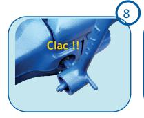
Correct positioning: Pin is correctly installed when you hear a "clac" sound informing of correct pin lockings.
