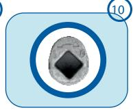
Correct locking (2): Once the pin has been correctly installed and locked, the pin should be in "head on top" position.
