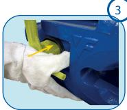
Sleeve insertion (2): We advise to use the TK13OD® to fully push the sleeve into its housing.
