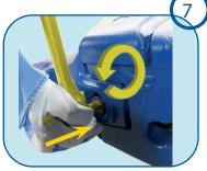
Pin clamping: Once the pin has been correctly installed, take TK13 OD® tool to screw the pin. Make sure to push the pin into the sleeve with the tool before screwing and then make a 180° counterclockwise pin turn.
