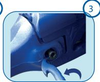
Pin removal: Using TK13OD® tool, remove the pin from the teeth/sleeve. You can also remove the pin manually.
