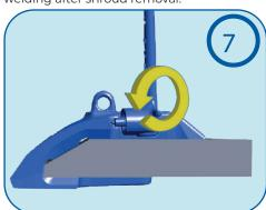
Pin clamping:: Re-assemble the shroud and pin on the adapter Once the pin has been correctly ins-
