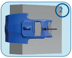
Pin removal: Using TK OD® tool, remove the pin from the shroud/sleeve. You can also remove the pin manually.
