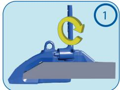
Pin unlocking: Remove the protective cap and insert the TK OD® tool into the pin, unlock the pin with a 180° clockwise turn.
