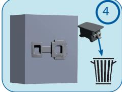
Shroud adapter cleaning: Clean up the shroud adapter and the pin housing. The adapter is ready to fitted with another new shroud.
