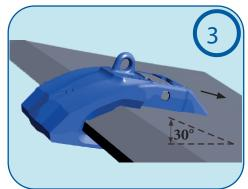
Adapter shroud positioning: Raise the blade edge to an angle of approximately 30°. Position the shroud assembly on the bade. Pull the adapter toward the center. Position adapter on blade, once the adapter is correctly located.
