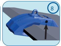
Protective caps installation: On both shrouds sides, insert the protective caps to avoid fines to fill up the pin hole.
