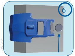
Welding instruction (step 3): We highly recommand to weld a Wear Button on each shroud sides (see above picture).
