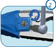
**Unpinning:** Once the TK D 3-9 clamping sleeve has been inserted into the pin head, unlock the pin by turning it counter-clockwise through 180°. Then lever out the pin with a screwdriver.
