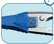
**Correct positioning**: Pin is correctly installed when the pin will be locked as shown.
