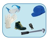
**Equipment**: The use of the TK D 3-9 tool is recommended for TURNKEY® Grizzly teeth assembly/disassembly. Always work safely and wear your safety equipment (hard hat, steel-toed shoes, gloves, safety glasses). Keep bystanders away.
