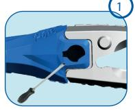
Removing protective caps: Before disassembling the pin, remove the protective cap using a flathead screwdriver, and clean any material in the pin head, so that the removal tool's appendix can be properly inserted into the pin.
