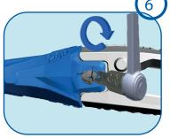
**Pin clamping**: Once inserted, take the TK D 3-9 clamping sleeve (installed on a square or ratchet wrench) and insert it into the key housing. Tighten and lock by turning 180° clockwise, while pushing in the pin.
