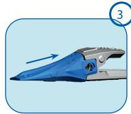
**Tooth assembly**: Install the TURNKEY® Grizzly tooth on the adapter.
