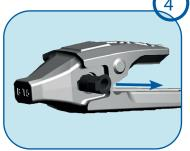
**Sleeve removal**: To eject the sleeve, take a screwdriver and extract it if it doesn't come out by hand.
