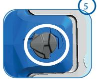
**Pin insertion (2)**: Before pin clamping, the pin should be in "head left" position. **Pin clamping**: Once inserted, take the TK D 3-9 clamping sleeve (installed on a square or ratchet wrench) and insert
