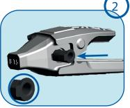
**Sleeve insertion**: Manually insert the sleeve. You will notice on the sleeve & the adapters some notches to make sure to respect the sleeve insertion direction.
