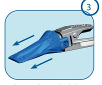
**Teeth removal**: Once the pin is removed, you can easily remove teeth
