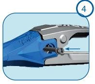
**Pin insertion**: Once the teeth is correctly installed on the adapter, insert the pin into the key hole while respecting the insertion direction (pin head left), then push it to the end.
