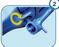
Pin unlocking: Once TK130D® tool is inserted into the pin, unlock the pin with a 180° clockwise turn.
