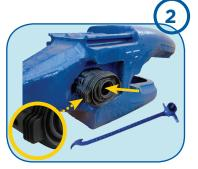
Sleeve insertion: Manually insert the sleeve. You will notice on the sleeve & the adapters some notches to make sure to respect the sleeve insertion direction. We now advise you to grab TK13OD® tool to proceed for installation.
