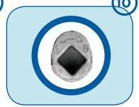
Correct locking (2): Once the pin has been correctly installed and locked, the pin should be in "head on top" position.
