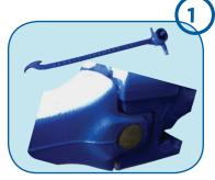
Protective caps removal: Remove both Left/right protective caps thanks to TK13 OD® tool.
