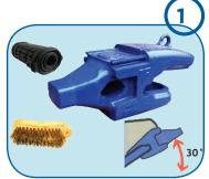
Cleaning: Tilt the bucket 30° upwards. Before inserting turnkey sleeve in its housing, we recommend to clean the adapter sleeve housing as well as the adapter nose to make sure the sleeve will be correctly positioned into the sleeve housing.
