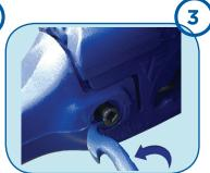
Pin removal: Using TK130D® tool, remove the pin from the teeth/sleeve. You can also remove the pin manually.
